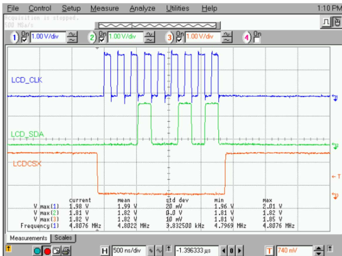
Figure 16: D/C bit set during each transmitted byte
